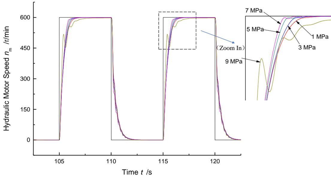
Fig.2 Response comparisons under different accumulator precharge pressure (600 r / min)
