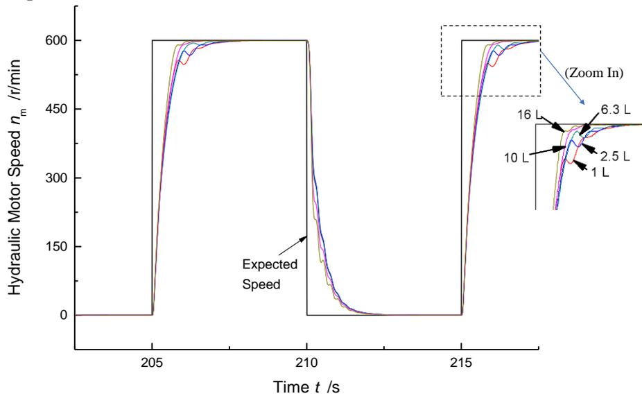
Fig.4 Response Comparison under different accumulator volumes (600 r / min)
