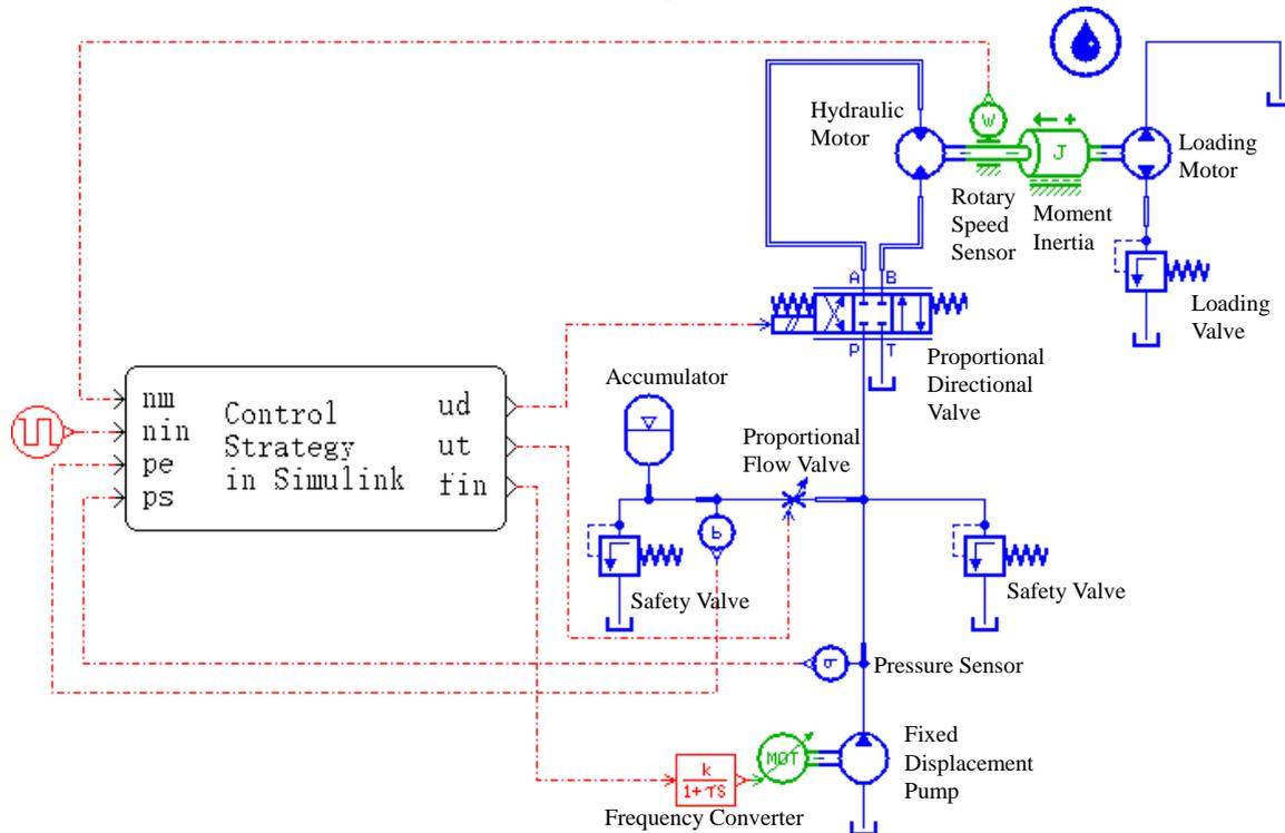
Fig.1 Simulation model of VCA in electro-hydraulic variable speed drive system
