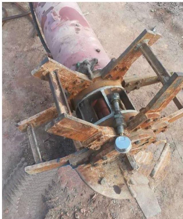
Figure 2 Mixing Head of Silt Solidification Machine
