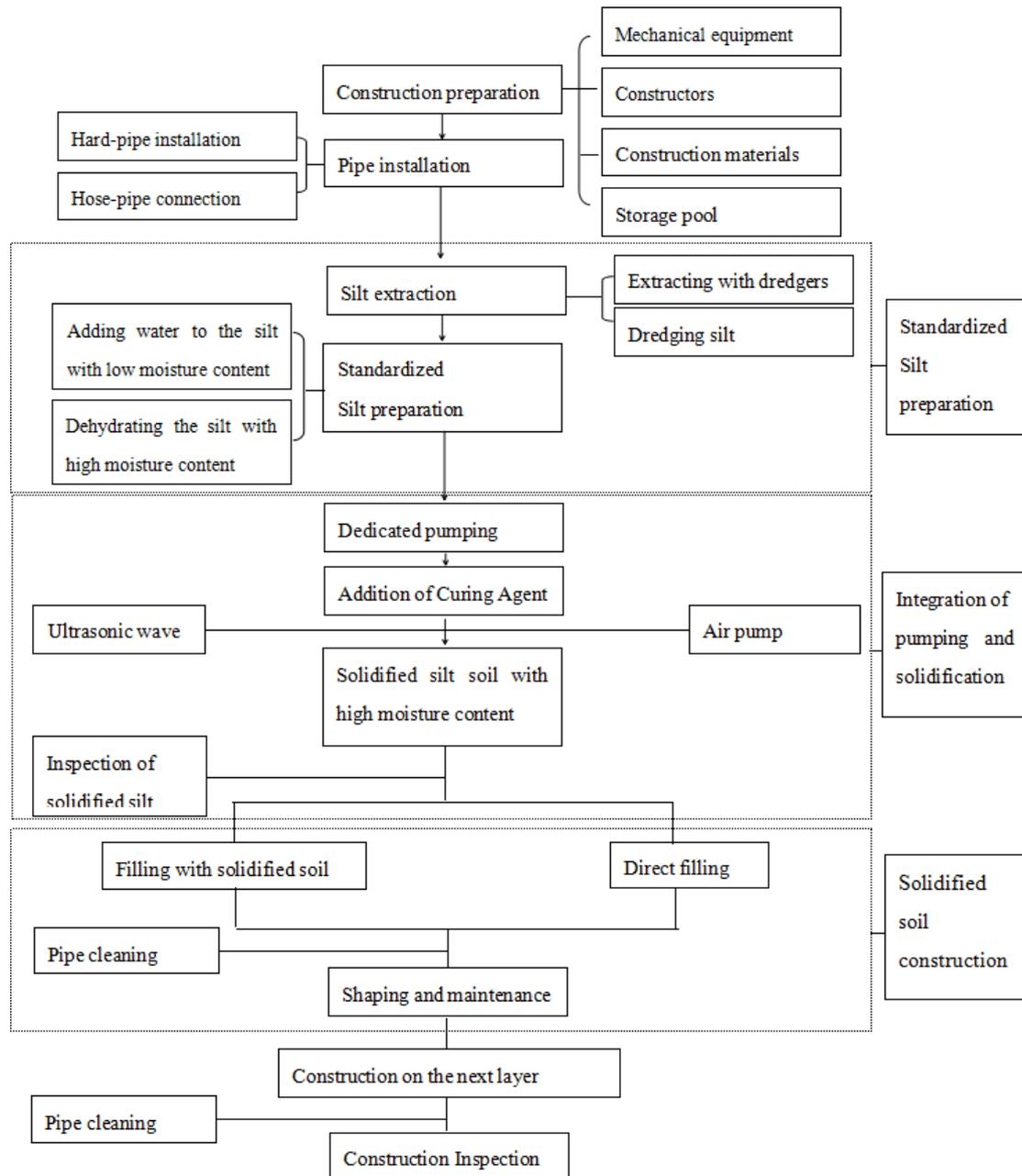
Figure 1 the Construction Process of the High Moisture Content Solidified Silt Soil
