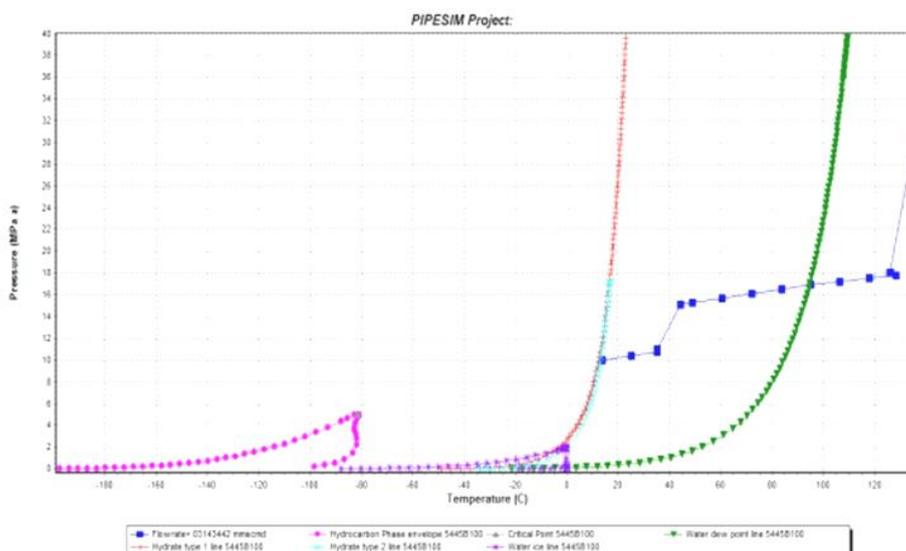
Figure 10. Pressure-temperature curve based on the phase diagram after throttling
