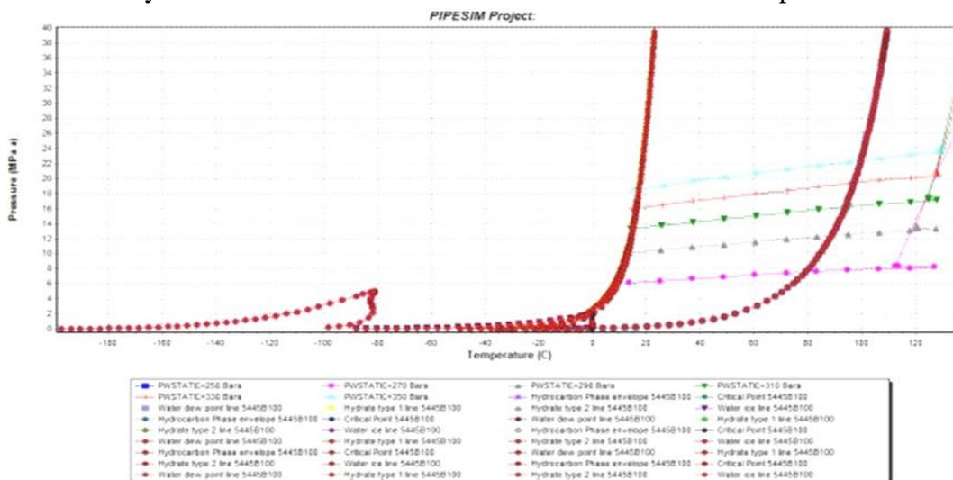
Figure 5. Prediction of hydrate formation in wellbore under different formation pressure conditions
