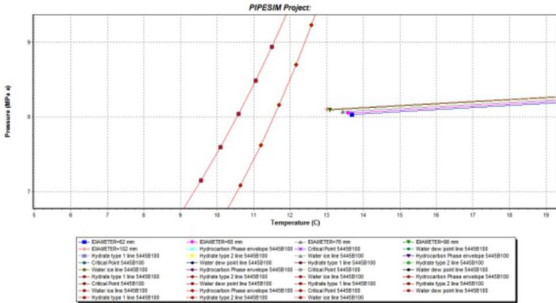
Figure 6. Prediction of hydrate formation in wellbore under different tubing size
