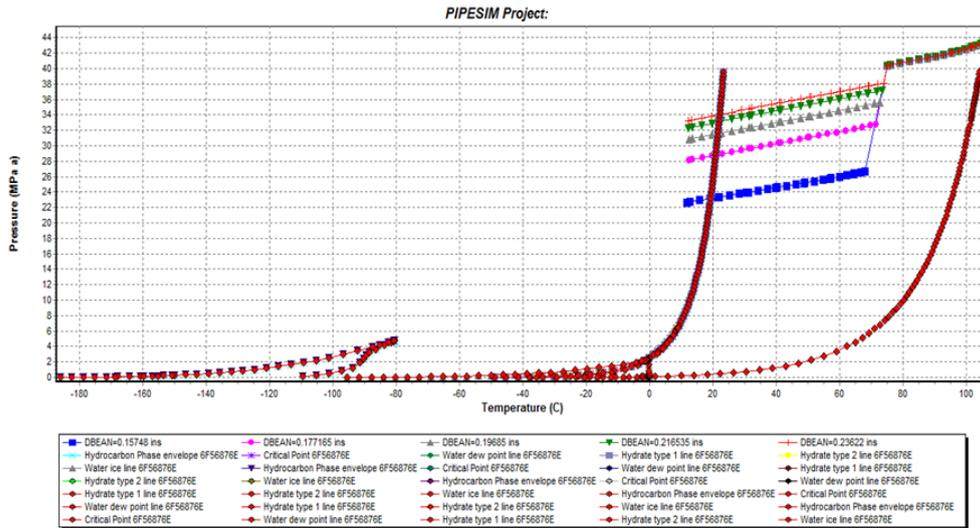
Figure 3. Hydrate formation temperature with different throttle diameters by using nodal analysis software
