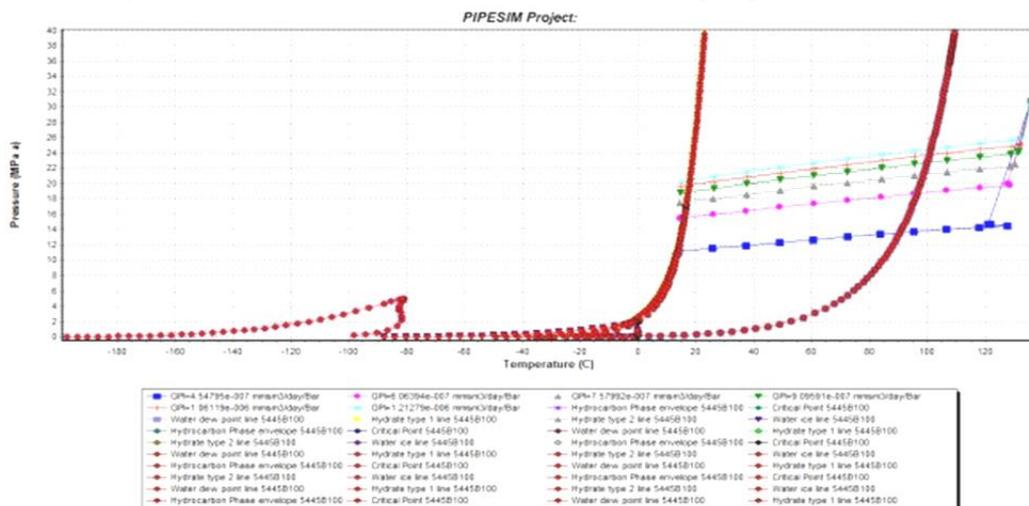
Figure 7. Prediction of hydrate formation in wellbore under different gas production conditions
