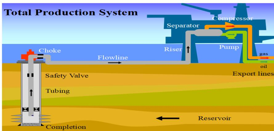
Figure 1. Producing system of natural gas well
