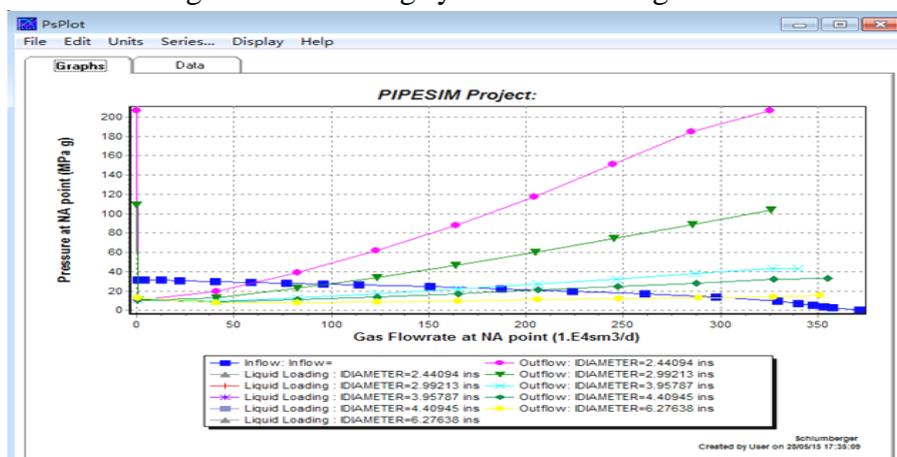
Figure 2. Drawing dynamic curve by using nodal analysis
