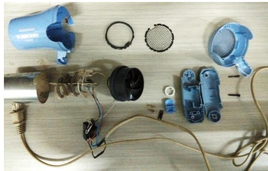
Fig.1 Explosion diagram of dismantling and blowing of blower
