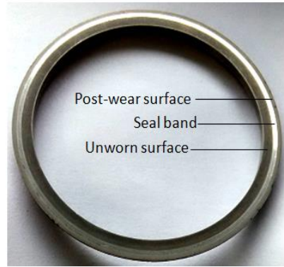
Fig.2 The wear condition of the stator
