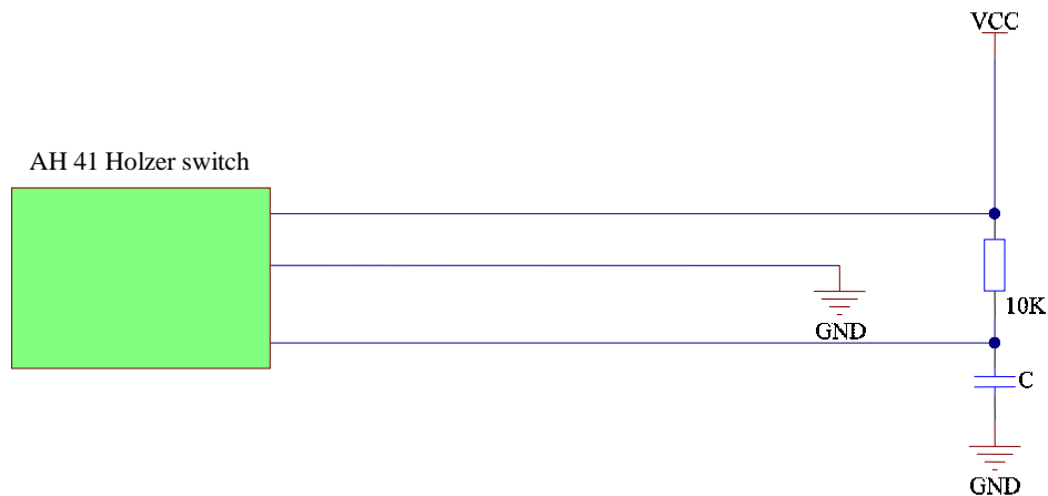
Fig. 2 Circuit diagram of the Holzer sensor
