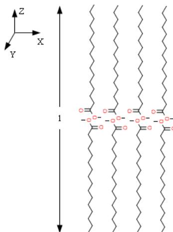
Fig.2 Stacking structure schematic diagram of C16:0 molecular
