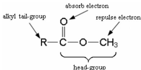
Fig.1 SFAME molecular structure schematic diagram
