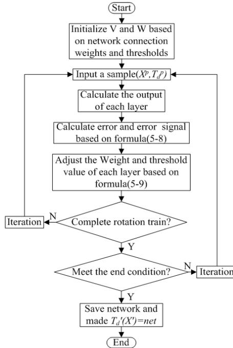
Fig.3 The gradient train procedure of BP neural network
