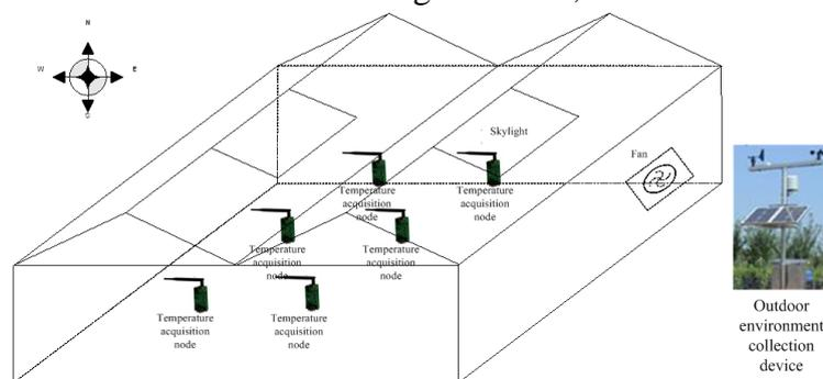
Fig.1 The schematic diagram of greenhouse structure and monitoring node distribution
