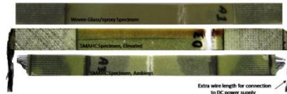
Fig. 13. Typical failed non-SMA reinforced composite specimen, and SMAHC specimens tested under ambient and elevated temperatures.
