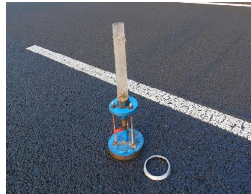
Fig.4 RIOH test device (in situ)
