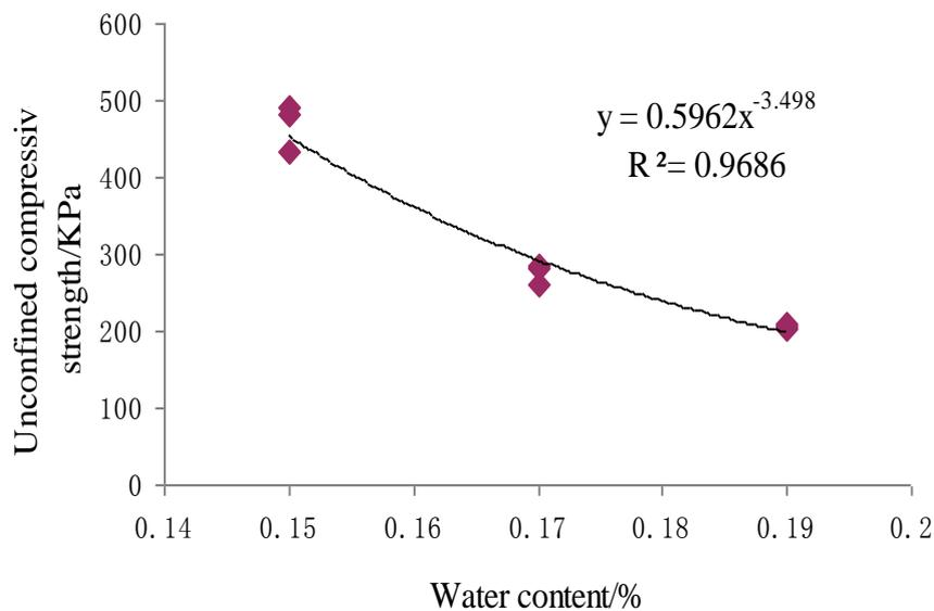
Fig.3 Water content-Unconfined compressive strength curve
