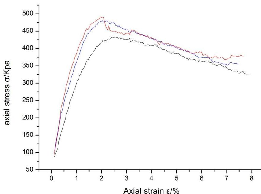
Stress-strain curve when  $\omega=15\%$
