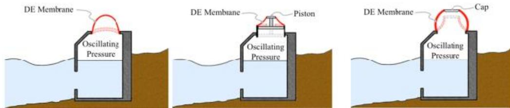
Fig. 1 Schematic diagram of possible realization of polymer oscillating water column
