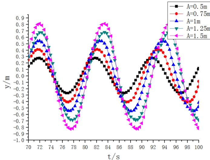
Fig. 4 curves of oscillating water column with wave amplitude
