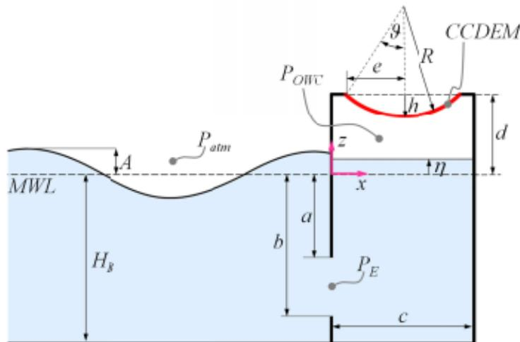
Figure 2. Model of polymer oscillating water column and related geometric parameter scheme
