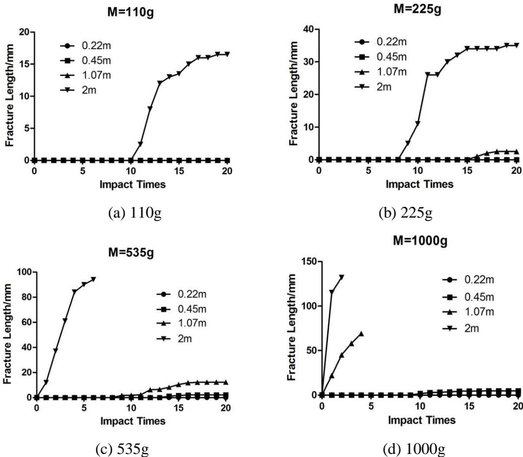
Figure 3. The crack accumulation of different mass falling balls under repeated impact
