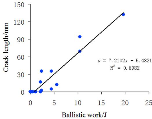
Fig. 2 Diagram of the development of crack under different impact work
