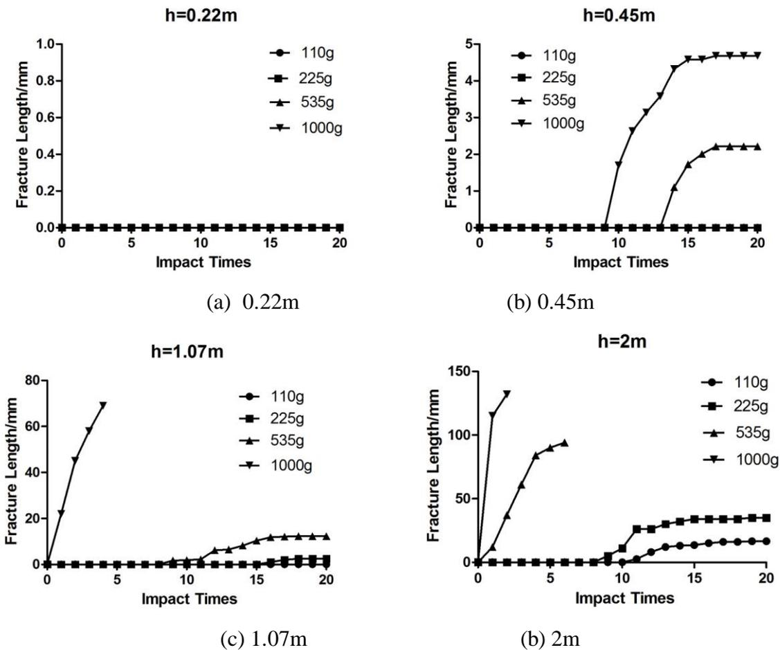
Figure 4. The cumulative development diagram of cracks at different heights under the impact of falling balls
