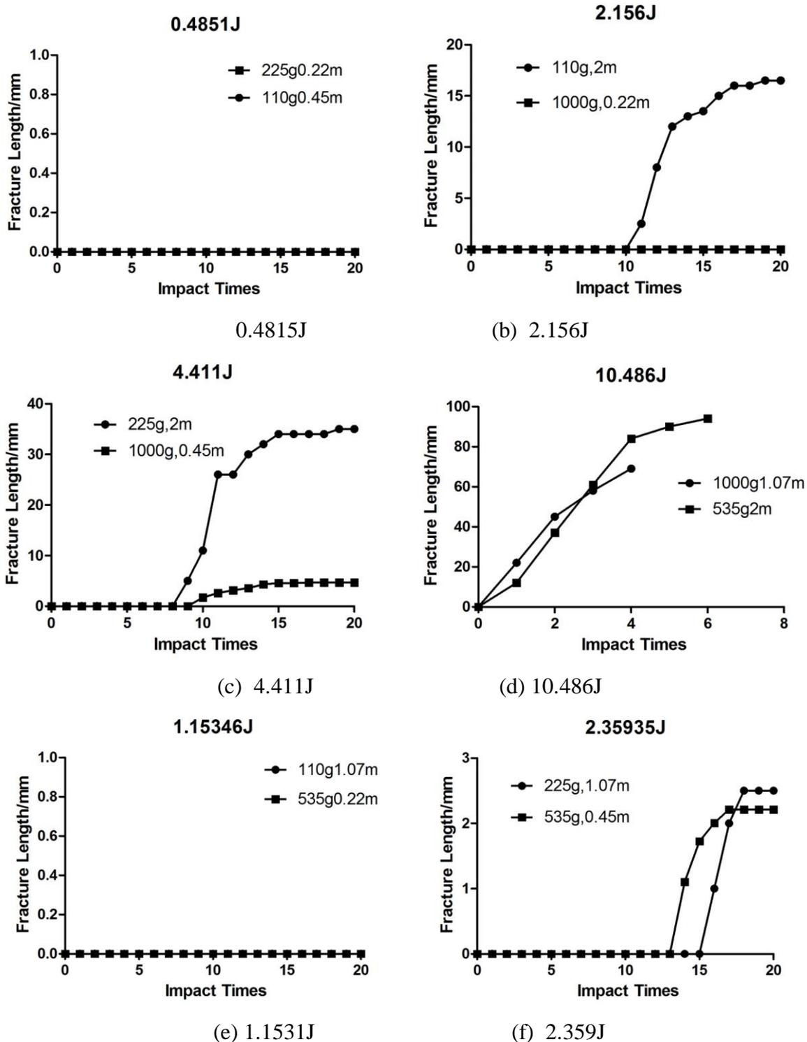
Figure 5. The diagram of crack accumulation development of different reasons under the same impact work.
