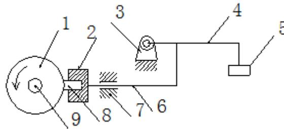
Fig. 1 Sketch of high temperature and high speed friction and wear test machine, 1- millstone, 2- sample rack, 3- hinge, call 4-, loading device, 5- counterweight, 6- transmission lever 7 fixing device 8 sample 9- power shaft
