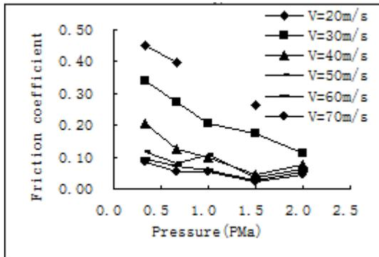
Fig. 4 Effect of pressure on friction coefficient
