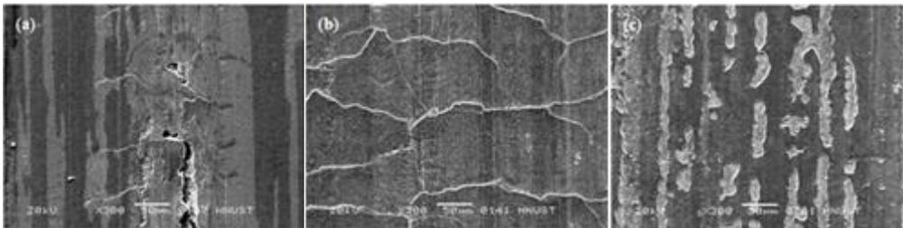
Fig. 7 SEM photos of worn surface of pin sample
