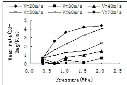
Fig. 5 Effect of pressure on wear rate
