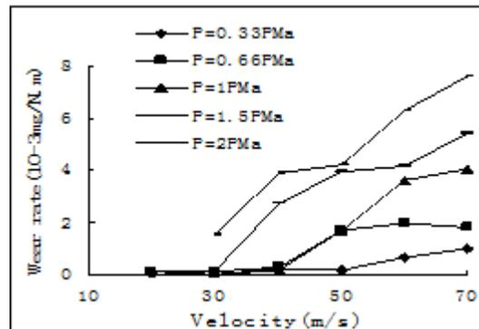
Fig. 3 Effect of sliding speed on wear rate
