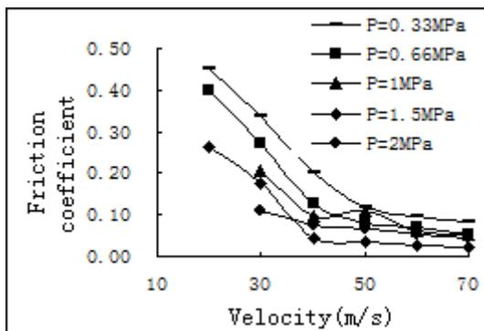
Fig. 2 Influence of sliding speed on friction coefficient
