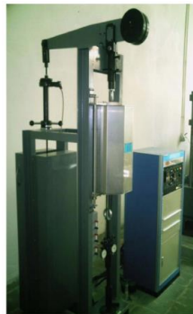
Fig 3. The Torsee creep and rupture testing machine.
