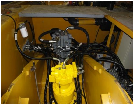
Fig.3 The Slewing mechanism of Excavator
