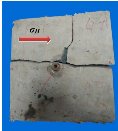
Fig.10 Re-fracturing fracture diversion of No.4 core
