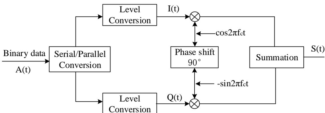
Fig. 2 The Block diagram of QPSK modulation principle
