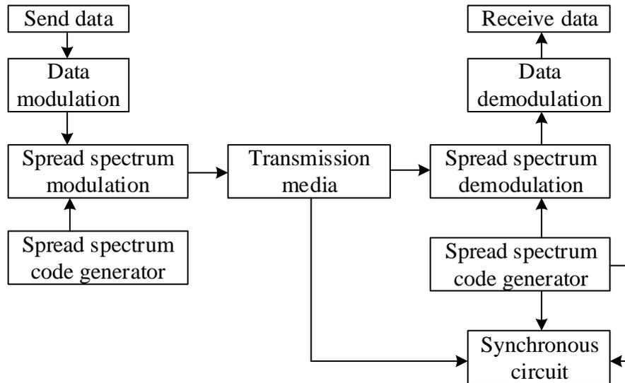
Fig. 3 DSSS principle block diagram
