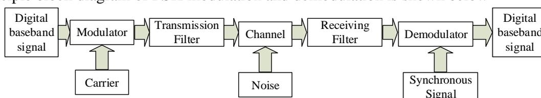
Fig. 1 The principle block diagram of FSK modulation and demodulation
