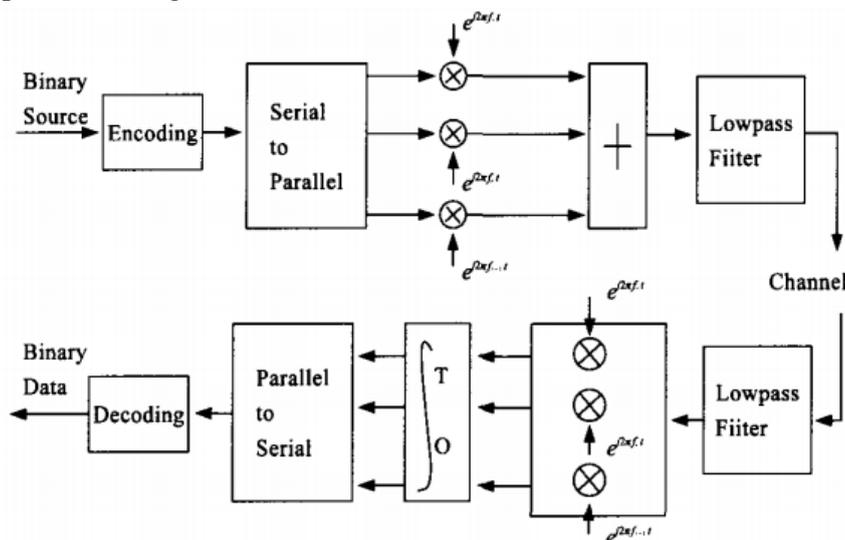
Fig. 4 OFDM principle block diagram
