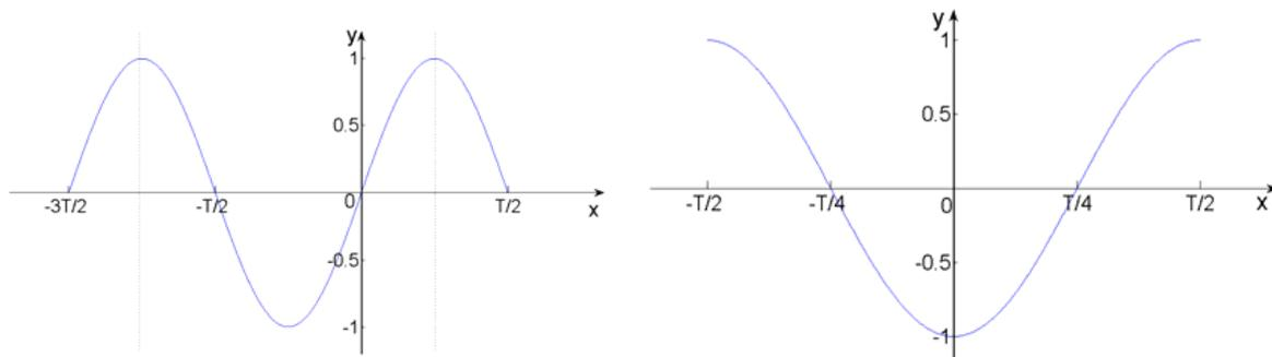
Fig. 5 Sinusoidal kernel function for detect pit defect
