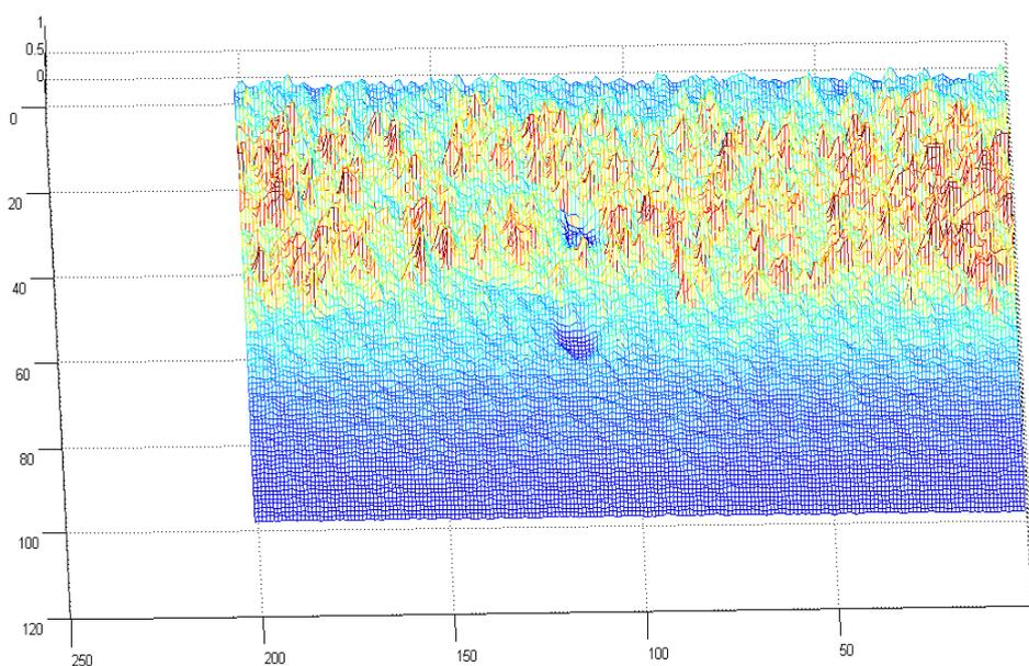
Fig. 4 Three-dimensional distribution of steel rod surface with pit defect
