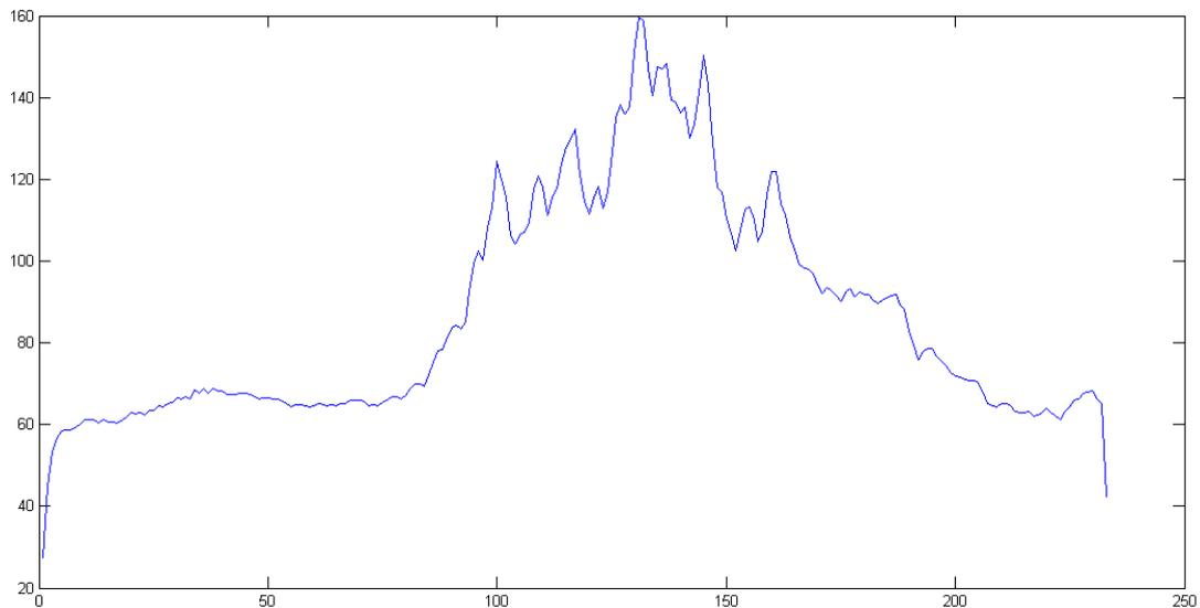
Fig. 3 Row pixel gray distribution of steel rod surface with no defect
