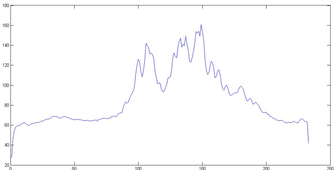
Fig. 2 Row pixel gray distribution of steel rod surface with pit defect
