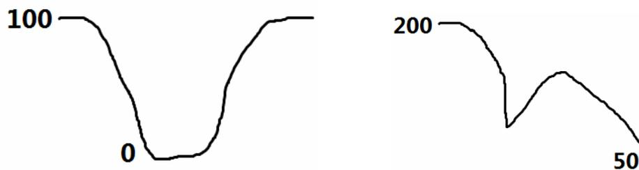
Fig. 6 Gray level situation of steel rod surface pit defect
