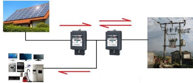
Fig.1 Smart distribution grid with PV system
