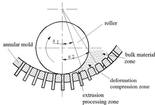
Fig.1 schematic diagram of the compression molding process
