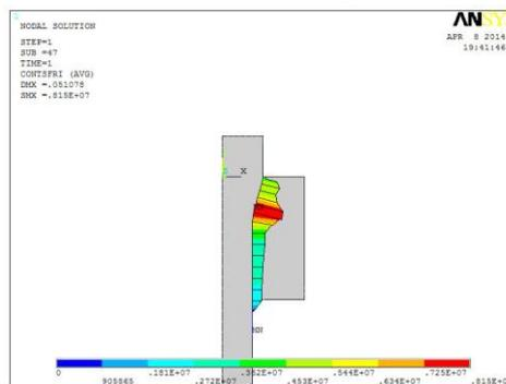
Fig.7 Friction stress chart of the straw in compressing process
