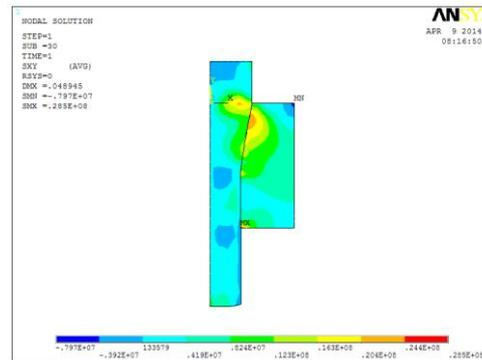
Fig.8 Shear stress chart of the straw in compressing process
