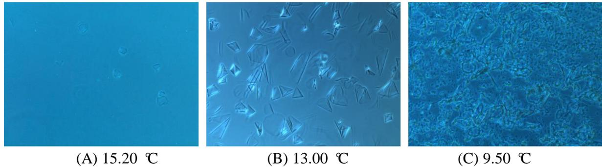
Fig.1 Microscope images of crystals of PME
