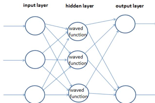
Fig1. the structure of wavelet neural network
