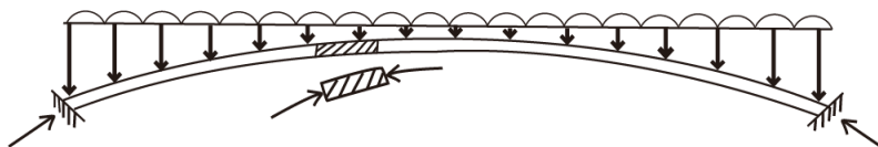
Fig. 2 the stress diagram of arch of the Zhaozhou Bridge
