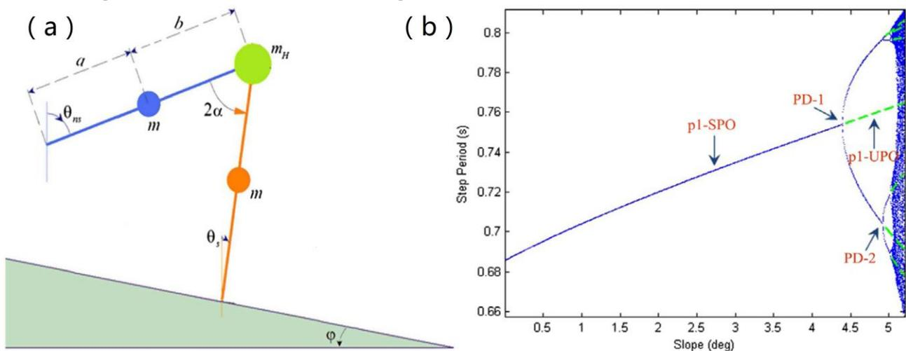
Fig. 3 Model of compass-like biped model (a) and its bifurcation diagram (b) [13]
