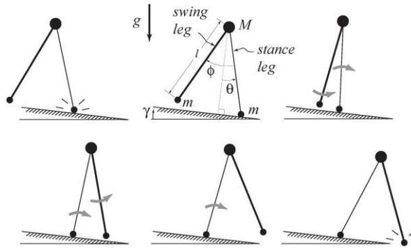
Fig. 1 A typical simplest passive walking step.  $\theta$  is the angle between the stance leg and the slope normal,  $\phi$  is the angle between the two legs,  $l$  is the length of the leg while  $M$  is the hip mass,  $m$  is the mass of the foot,  $g$  is the gravitational acceleration and  $\phi$  is the slope angle [11]. Adapted from Garcia et al.
