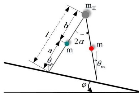
Fig. 2 Model of a compass gait biped robot on a slope. The robot consist of two knee-less legs, each having a joint mass and a third point mass coincides with the hip joint [12].
