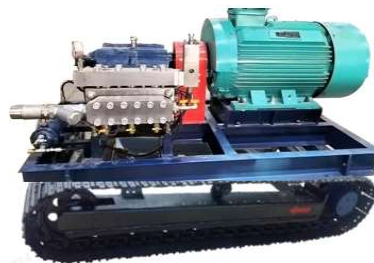
Figure 1. Fracturing pump set
