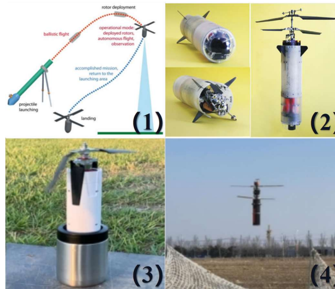
Fig. 6 Single axis rotor catapult launched foldable drone
