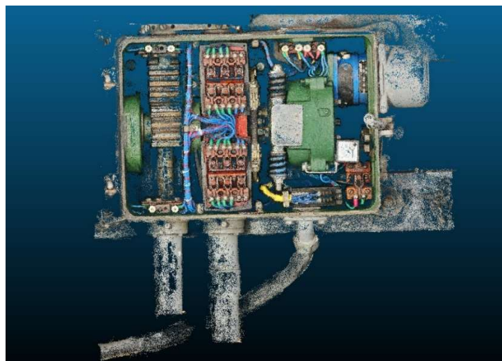
Figure 5. Dense point cloud reconstruction of switch machine
