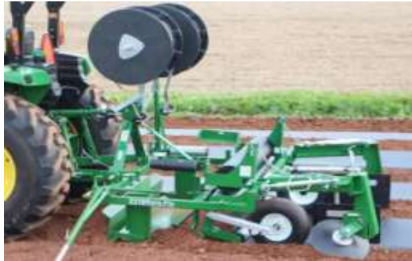
Fig. 7 Rain-FloIrrigation (USA) Company 2370 ridging mulch machine overall picture
