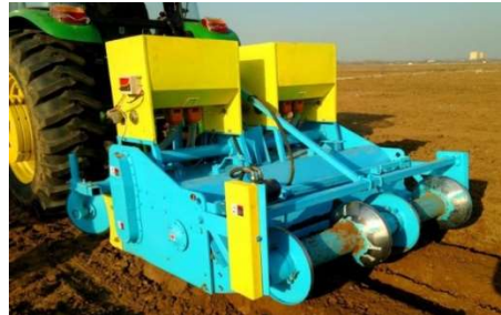
Fig. 2 Model YS-1GVFM-125A Fertilizer Mulching and Mulching Machine
