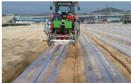
Fig. 5 KOMACHINE (Korea) KG-PH9000 seeding and laminating machine
