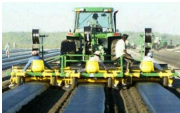
Fig. 8 BP480 model ridging and mulching machine
