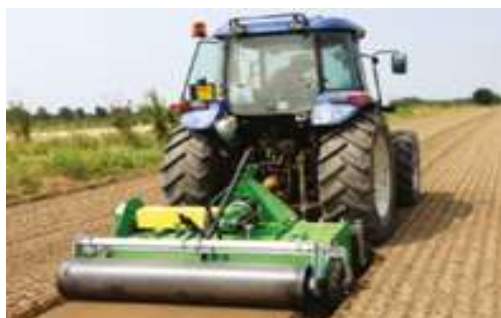
Fig. 6 HORTECH (Italy) PERFECTA-140 vegetable planter ridger
