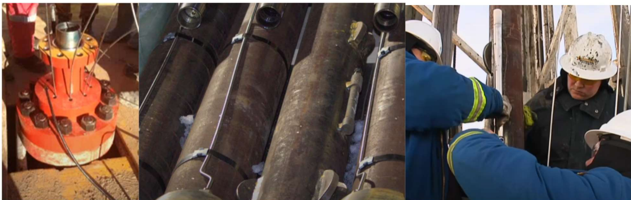
Figure 3. (a) Customed wellhead (b) Customed Joints (c) Example of casing-conveyed downhole gauge Installation
