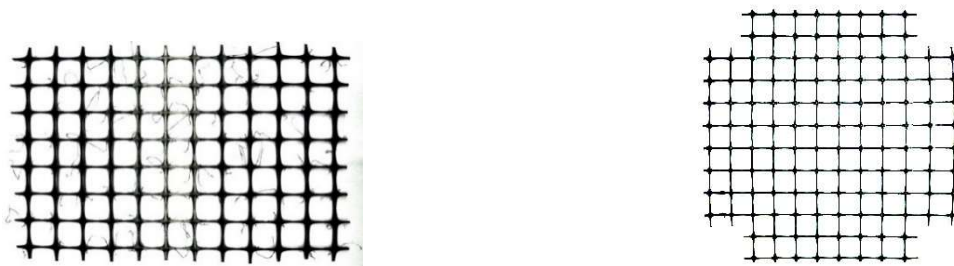
(a) The geogrid specimen without side restraint (b) The geogrid specimen with side restraint
