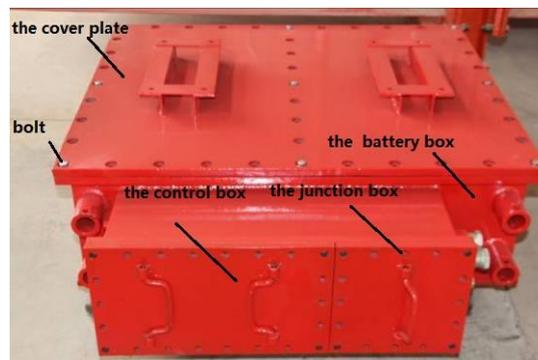
Fig 1 8t Mine-used electric locomotive power box
