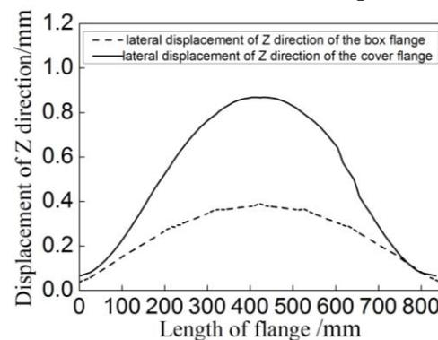
Fig 4 The lateral displacement of Z direction of the box and cover flange
