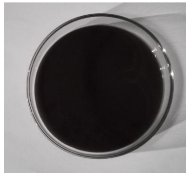
Fig. 1 MR fluid samples
