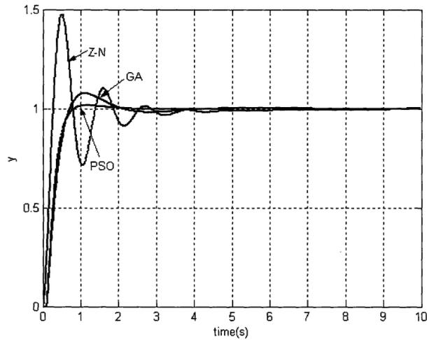
Fig.1 The unit step response curve of three kinds of tuning results of the object  $G_1$
