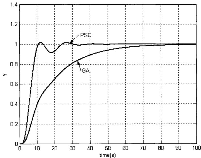
Fig.5 The unit step response curve of the two tuning results of the object  $G_2$
