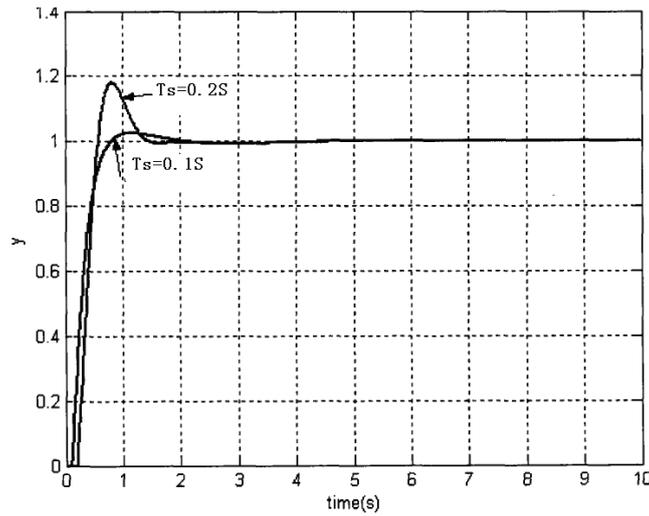
Fig.3 The unit step response curve of object  $G_1$  before and after the time delay variation
