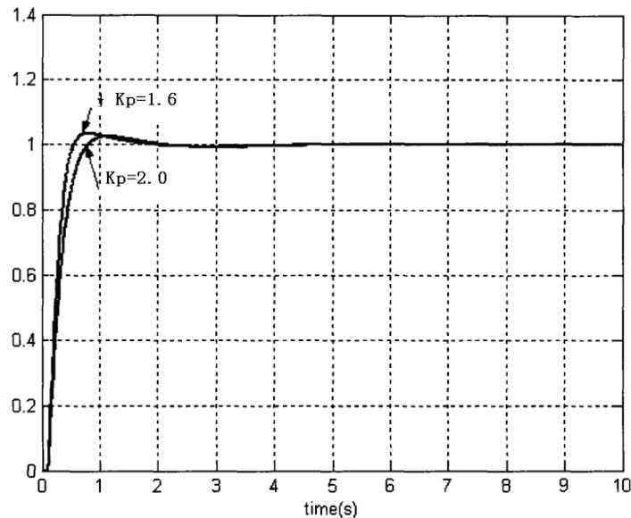
Fig.2 The unit step response curve of the object  $G_1$  before and after the gain change
