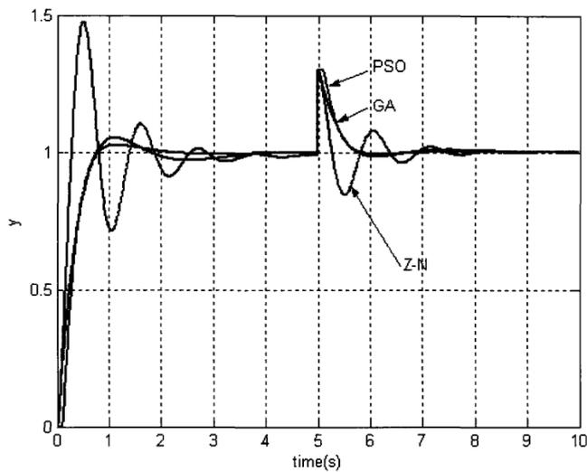
Fig.4 The unit step response curve of the object  $G_1$  is disturbed
