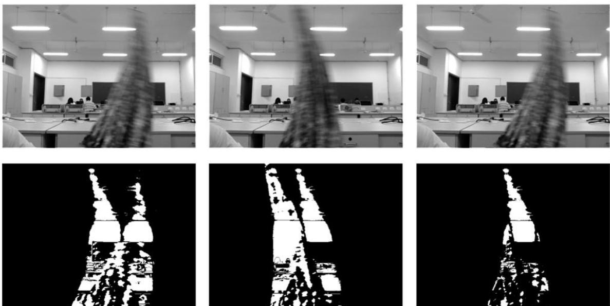
Figure 1 The moving object detection of frame difference method
