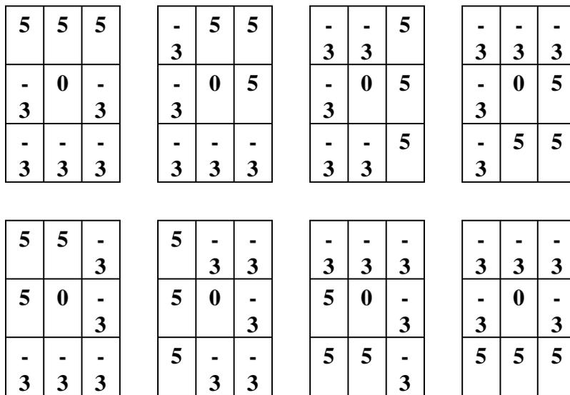
Figure 3 8 filter templates for Kirsch edge detection
